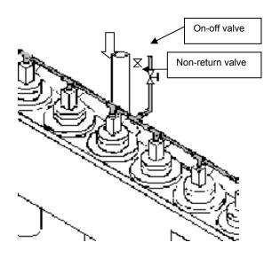
The pilot air for the solenoid is taken from the incoming tube to the pressure tank. The pipefpr the pilot air is common for all valves in one tank and is connected upstream the main on- off valve of respective tank.
